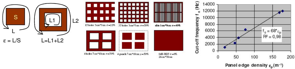
a. Edge density  $\epsilon$       b. Scale models measured      c. Measurement trend  $F_c = 68 \cdot \epsilon$
