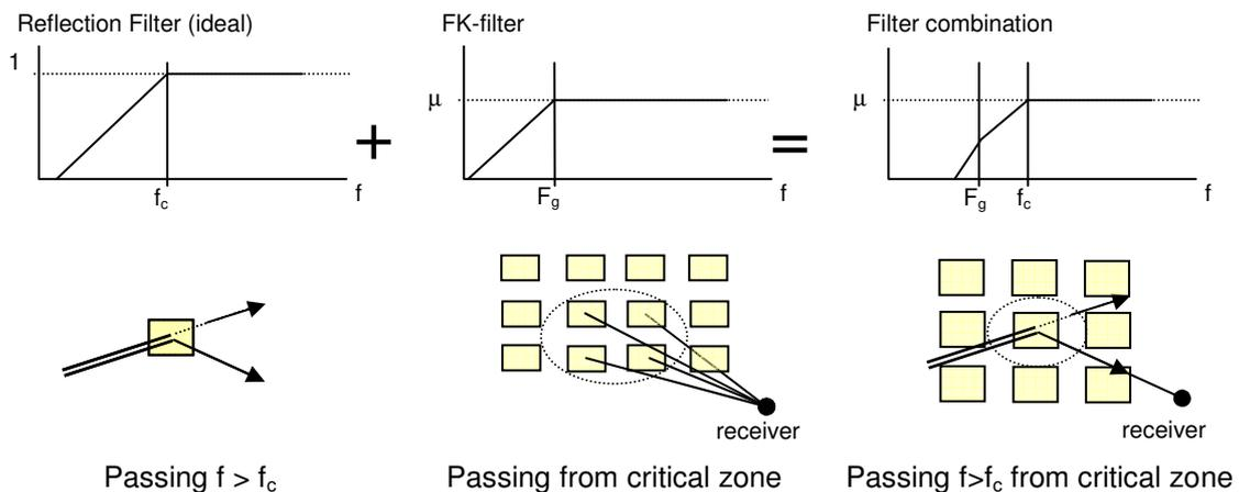
Figure 1. Serial combination of two filters
