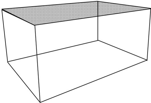
Figure 1 The hard case. Only ceiling is absorbent.
