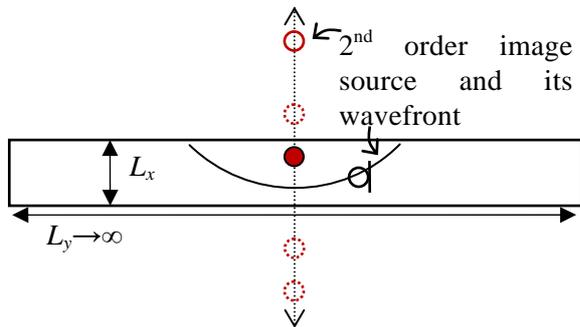
Figure 2 Axial mode study. x-y-plan of virtual cuboid, hard, test room with  $L_y$  and  $L_z$  approaching zero, containing source (red dot) and a receiver collecting wavefronts from axial image sources.
