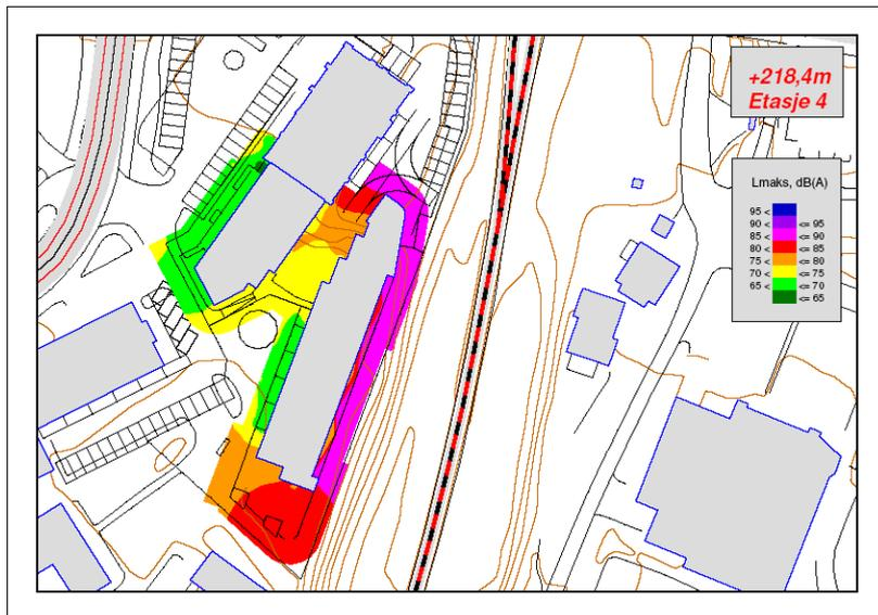
**Figure 4,** noise levels on façade, given as  $L_{Amax}$
