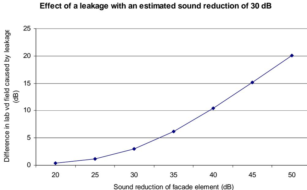
**Figure 4:** Calculated difference between the given laboratory value for the glass façade and the expected influence of a leakage with  $R_{\text{leakage}} = 30$  dB.
