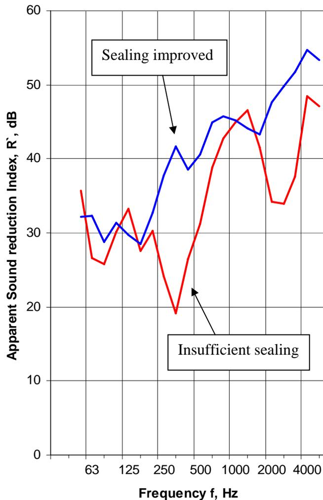
**Figure 2:** Measurement performed on the same glass façade before and after sealing improvements.
