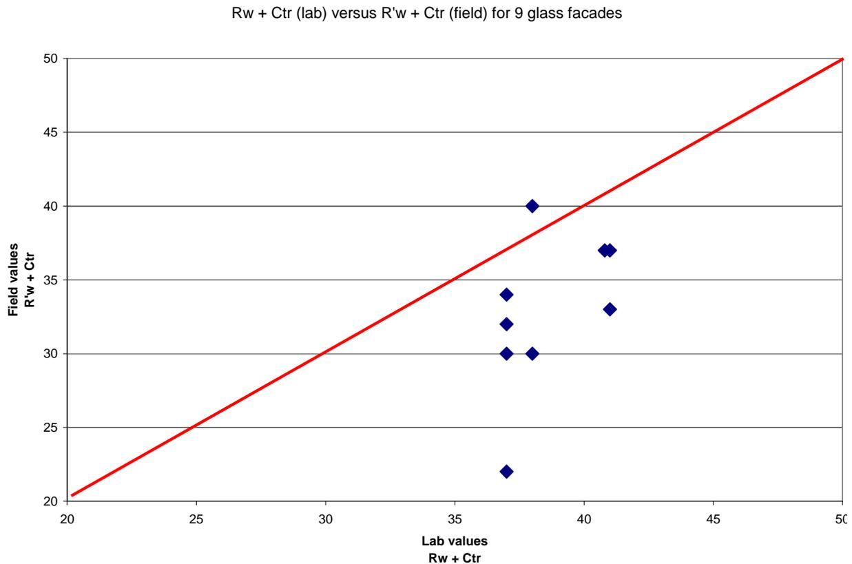
**Figure 1:** Measurements performed on 9 glass façades. Results are shown as the sound reduction index  $R'_w + C_{tr}$ .
