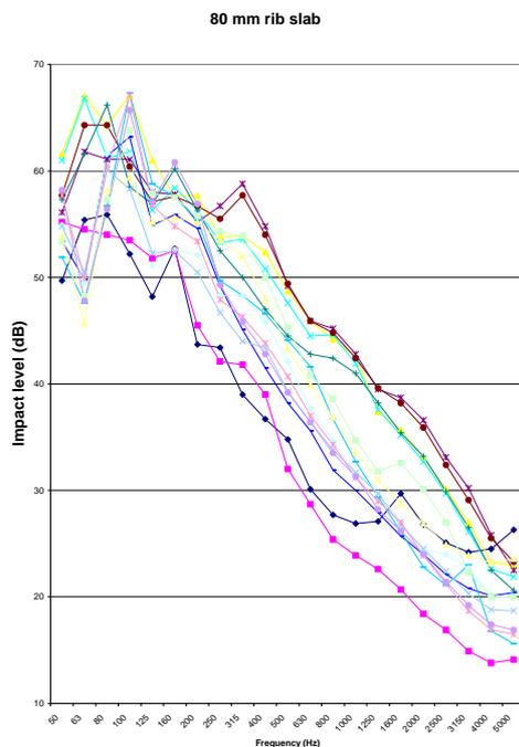
It seems that plotting field measurement results for different types of impact absorbing materials for use under a parquet floor give a very confusing picture. Our analysis gives us three possible conclusions so far:
